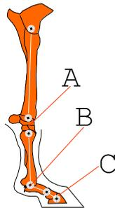
**Figure 3.** Definition of the angles: hoof, C; fetlock, B; and carpal, A, joints, the small dots are reference points monitoring the movements of the different joints.
