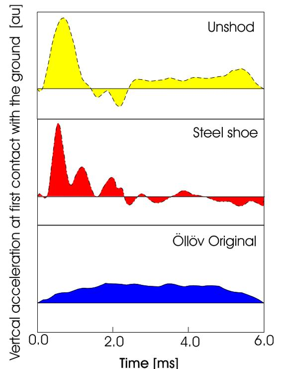
Figur 2. Results for the vertical acceleration of the hoof at first contact with hard ground, Drevemo and Johnston 1992.
