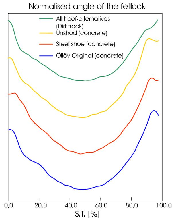
**Figure 5.** Normalised angle of the fetlock during the stance phase. The different shoe alternatives relate to hard ground.
