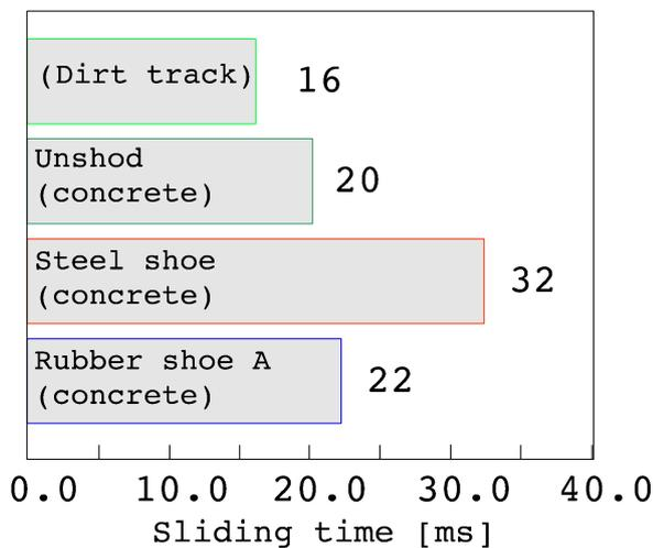
Figur 1 Sliding-times for the different shoe alternatives and surfaces, measured by Drevemo and Johnston (1992).
